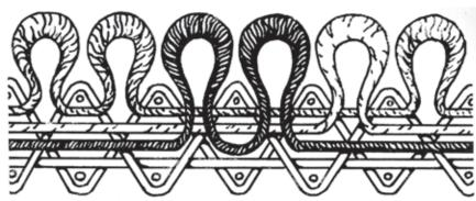
Diagram of the construction of a Brussels carpet.
