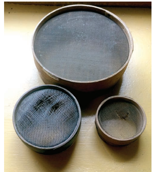
Large brass wire drive and two small horsehair drives.
