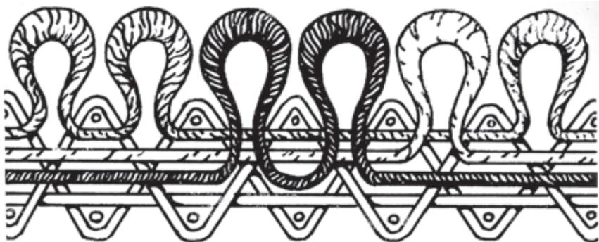
Diagram of the construction of a Brussels carpet.
